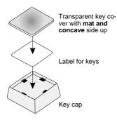
Each key should be labelled individually. You can use the empty labels delivered with the system to do so.
